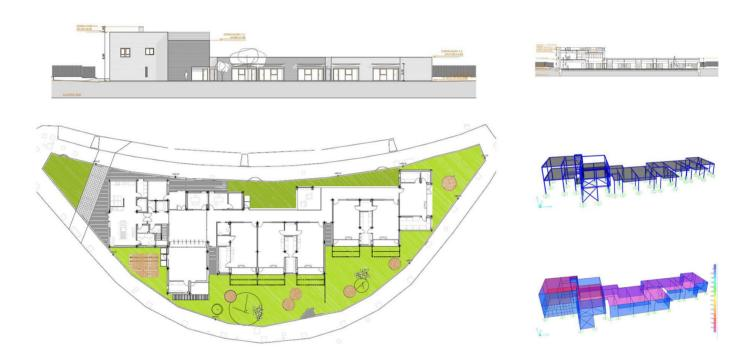
The planned building is located on a plot with a surface area of  $1,509 \text{ m}^2$ . It is a ground and ground floor building consisting of 6 units of children's classrooms, a multi-purpose room and a library. Both the classrooms and the common areas are equipped with large glass surfaces to provide natural light. All the classrooms have an outdoor patio, semi-covered by an outdoor porch that provides shade for the play area.
